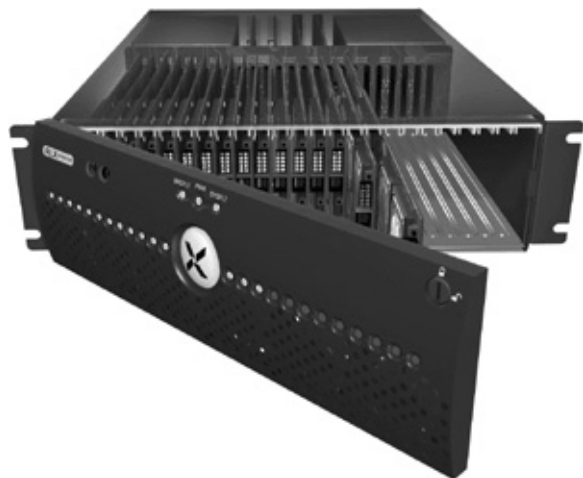
Figure 4. One 24-Node Chassis from Green Destiny
